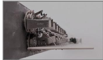
Board mounts on jack sleeve lugs and at right angle to panel.
